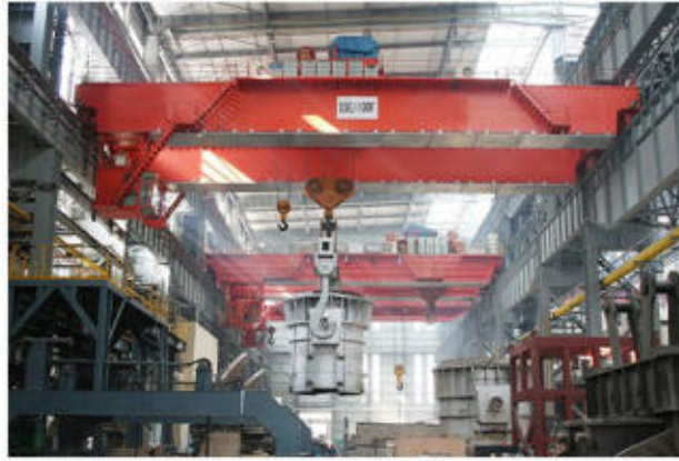
CASTING OVERHEAD CRANE
