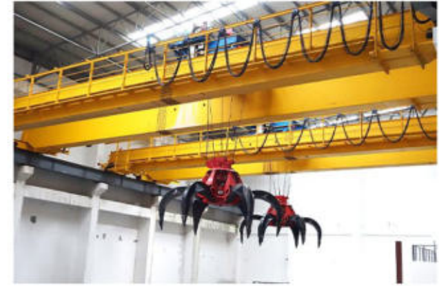
QZ GRAB OVERHEAD CRANE
